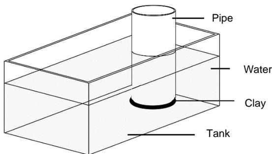
The demonstration is more effective if a circular ribbon of clay or Blu Tak™ is used as a seal between the pipe and the base of the tank – but this is not essential.
