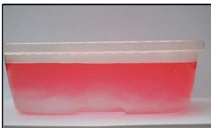
Near-boiling water, coloured with washable red paint, added to the left of the lunchbox – flowing along the top from left to right.
