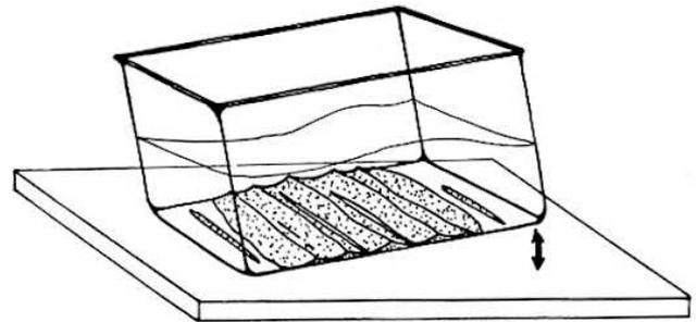
Gently lift one side of the container up and down, as illustrated in the diagram opposite, until the sand has formed a pattern on the base of the container.
