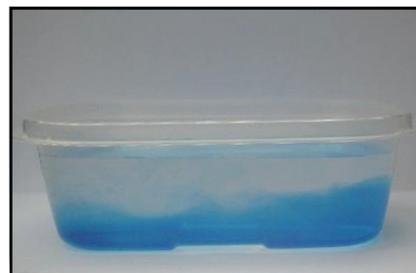
Iced water, coloured with blue food colouring, added to the left of the lunchbox – flowing along the bottom from left to right.
