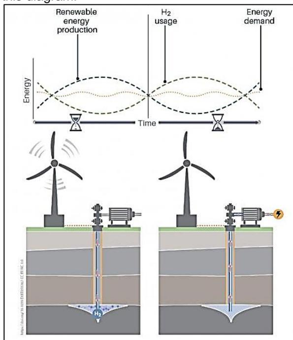
The graph shows that as wind increases, the turbine adds energy to the national grid until demand is reached. After that, the extra energy is used to generate hydrogen which is stored underground. Later, when the wind drops or the turbine is shut down, the stored hydrogen is burnt to generate electricity. This evens out the energy supply, shown by the dotted yellow line on the graph.
