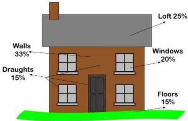
Heat loss diagram for a typical house (% figures rounded up)
