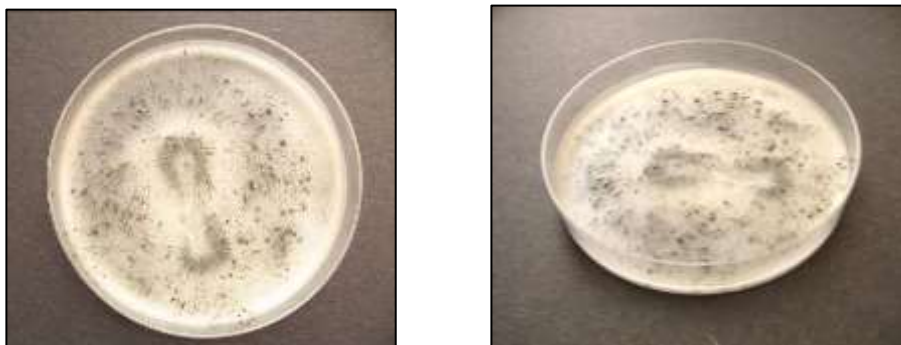
'Petri-dish magnetic field preserved in iron filings in wax' (Michèle Bourne, ESEU)
