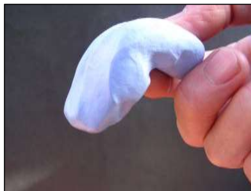
Bend it (plastic deformation)
