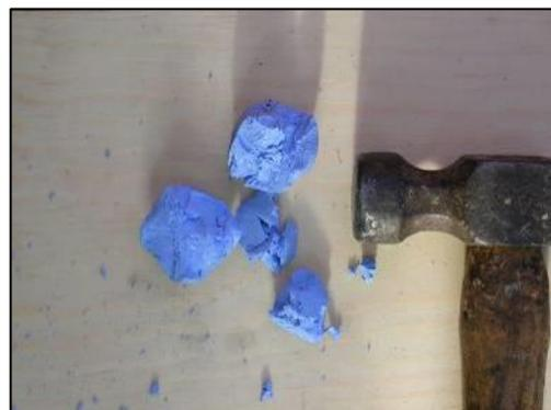
Shatter it (brittle deformation)
