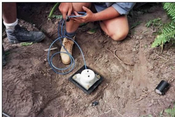
Tilt meter in use in Montserrat
