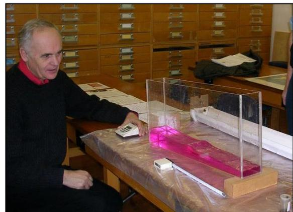
Modelling a tsunami in a wave tank
