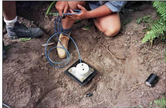
Tilt meter in use in Montserrat
