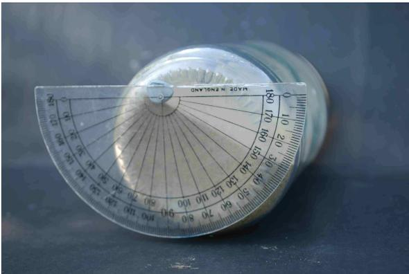
How to measure the angle of rest of dry sand. (Note: It is easier to use the protractor as shown, with the 90° line running vertically, than with the zero line of the protractor resting on the table top).
