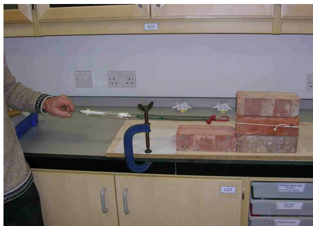
The brick 'earthquake' in action – b) Using a Newton meter to quantify the forces involved. The front brick is stopped from sliding by a board, held to the bench by a clamp. (Photos: P. Kennett)
