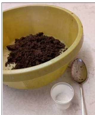
Fig 1. Bowl with 500g soil, measuring beaker containing water and metal spoon
