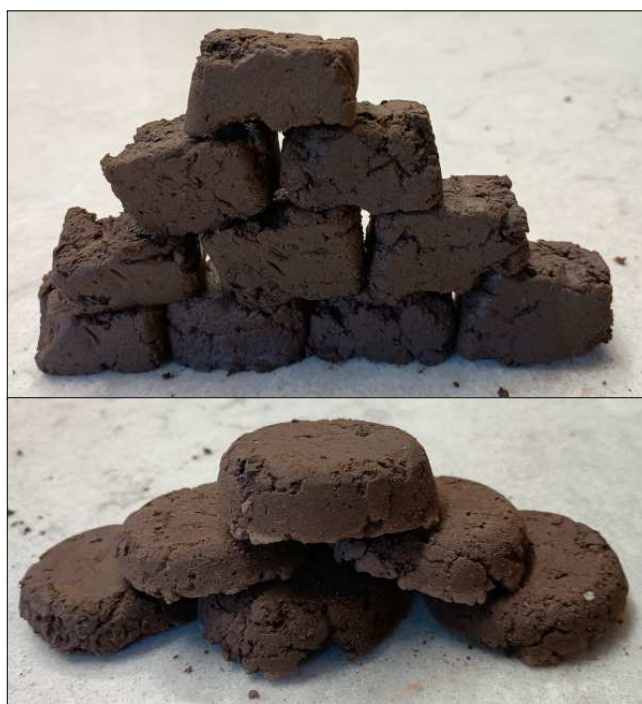
Fig 4. The finished bricks - as you can see, we needed to remove more air and smooth the tops more evenly! Photos Elizabeth Devon
