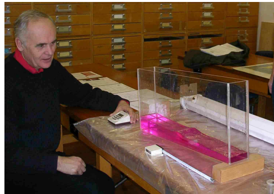
Timing the flow of a tsunami in a plastic tank (Photo: P. Kennett)
