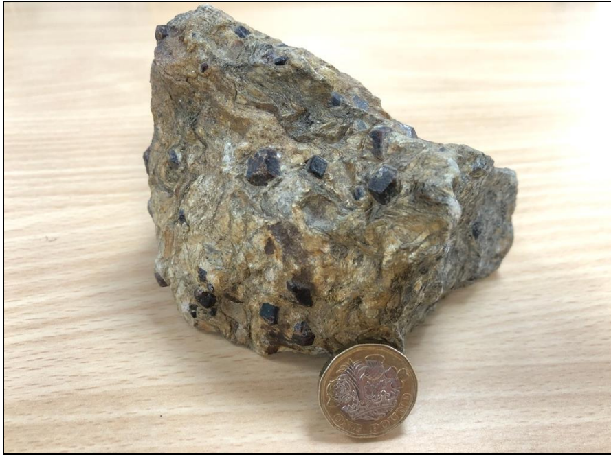
Fig: 1 Example of a garnet mica schist specimen suitable for tactile interpretation. The weathering of the surface has left euhedral garnet crystals protruding. The shape of these can be determined by touch and used to identify the mineral and an interpretation can be made independently by a student with VI.
