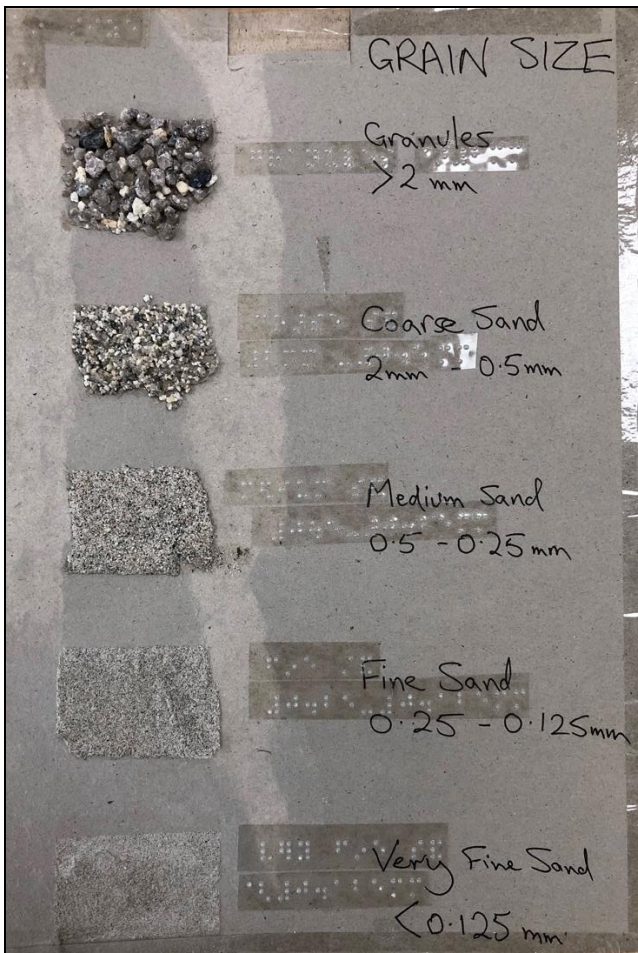
Fig: 3 A tactile grain size card made from sieved sand, thick card and PVA glue. The labels are made from self-adhesive braille strips, the writing was included to help the practical assistant. The tape around the edge of the card was added to make it durable enough to last the duration of the course. (Photo: M. Walsh)
