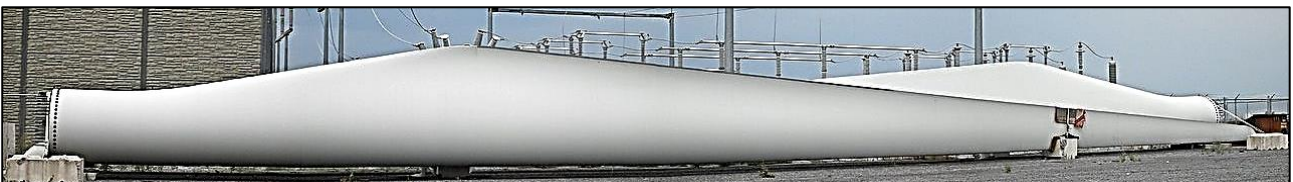
A 50 metre-long wind turbine blade. Blades three times this size are currently being manufactured; blades five times larger (250m length) are in prospect (by Z22 CC BY-SA 3.0).
