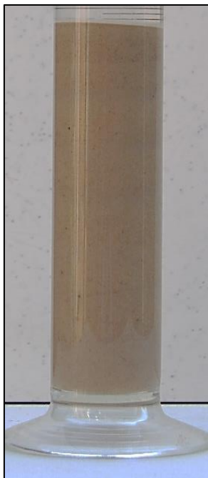
Several beds of sediment in a measuring cylinder, but the bedding planes cannot be seen because the sand is all the same colour. (Chris King).
