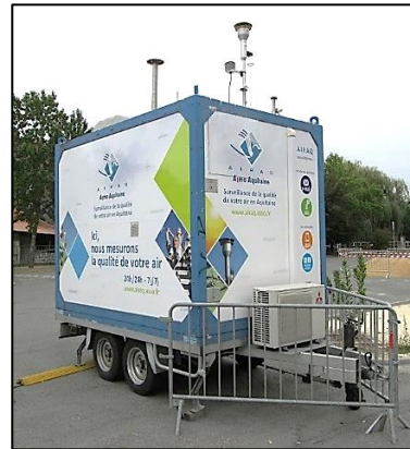
An air quality measuring station in France.
