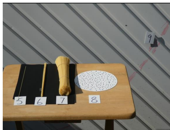
A demonstration of “earthquake energy” using spaghetti, showing one strand (barely visible), 30 strands, 900 strands, a circle of card representing the ends of a bundle of 27,000 strands and part of a 2m diameter circle on a garage door, representing the ends of 810,000 strands. (Photo: P. Kennett)
