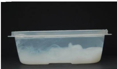
Milk added to the left of the lunchbox – flowing along the bottom from left to right.
