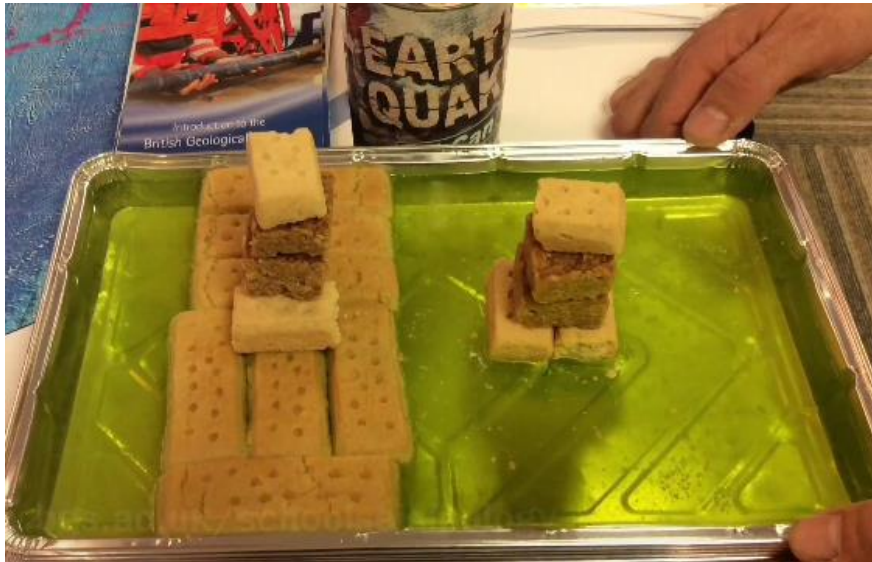
The jelly/biscuit model used to demonstrate seismic site amplification (video - http://www.earthlearningidea.com/Video/Mexico_City.html ) (Photo and video copyright Paul Denton BGS creative commons.)
