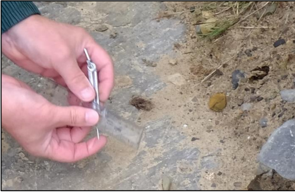
The method using a pair of compasses and a ruler to measure the depth of glacial striations, Traeth Bychan, Anglesey, UK. (Peter and Maggie Williams).
