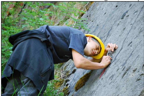
Measuring angle of dip on tilted rocks. (Peter Kennett).
