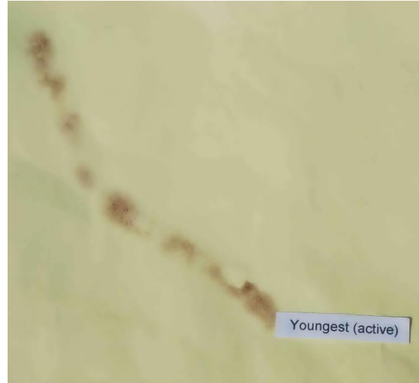
Fig 2. The result of moving a card over a candle flame as shown in Figure 1 (Photo: Peter Kennett)
