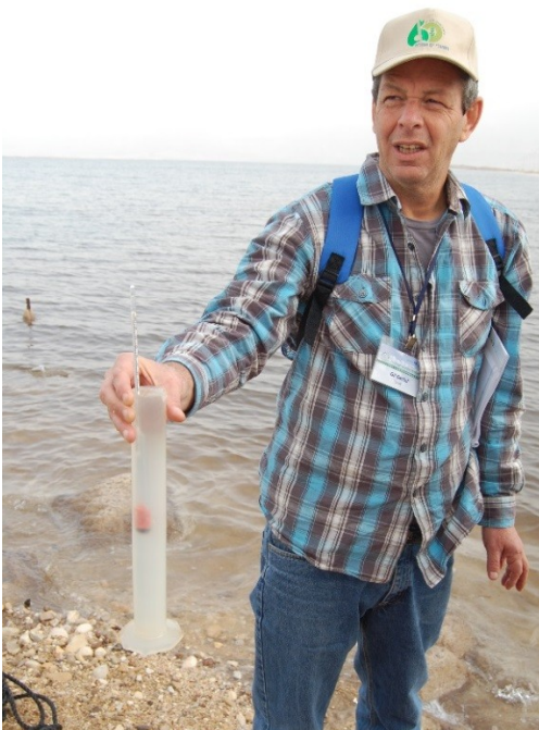
A scientist measuring the density of the salty water of the Dead Sea to find out how much more evaporation is needed before salt will crystallise from the solution. (Photo: Chris King)
