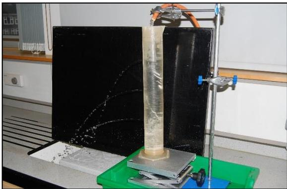
Turn on the tap to fill the cylinder and then maintain a constant head. Jets of water will squirt out of the hole under different pressures. The photo shows the lower jet squirting further and with a shallower arc than the upper one, indicating how hydrostatic pressure increases with depth in the cylinder.
