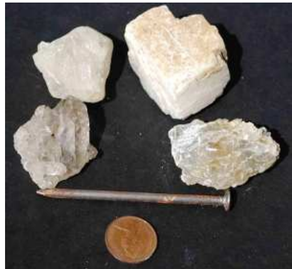
Hardness: fluorite, calcite, gypsum, quartz with a steel nail and a 'copper' coin
