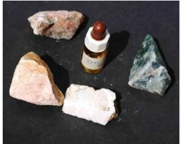
Acid test: gypsum, fluorite, calcite, barite and a dropper bottle of dilute hydrochloric acid
