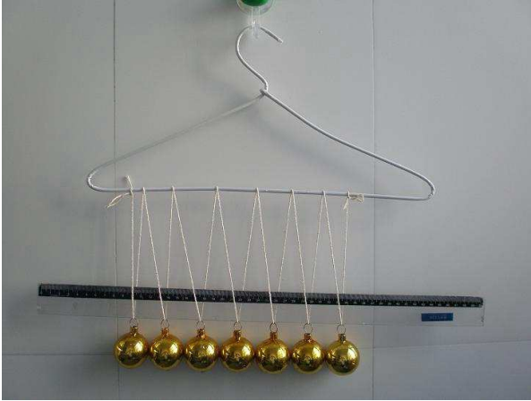
Aligning balls in a “Christmas style” wave transmission model with the aid of a ruler.
