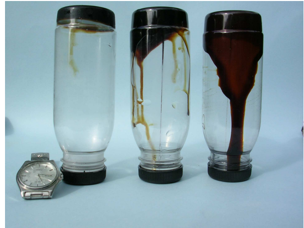
Treacle at three different temperatures, where the containers have been inverted at the same time (Photo: P. Kennett)
