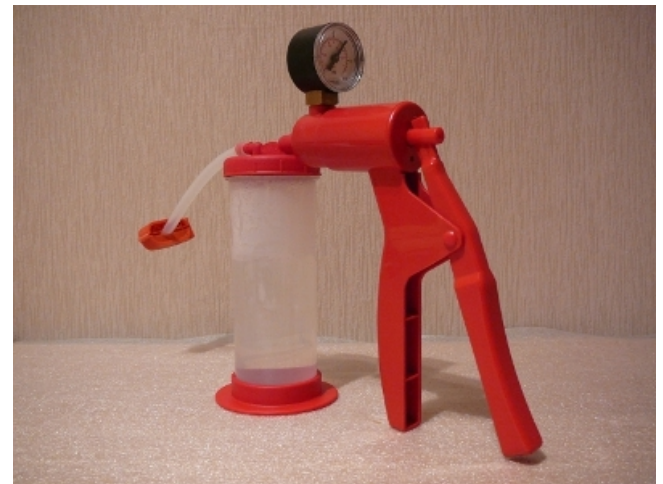
Figure 2: Water boiling below 100°C under reduced pressure of vacuum pump
