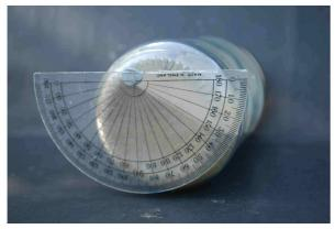
How to measure the angle of rest of dry sand. (Note: It is easier to use the protractor as shown, with the  $90^{\circ}$  line running vertically, than with the zero line of the protractor resting on the table top).
