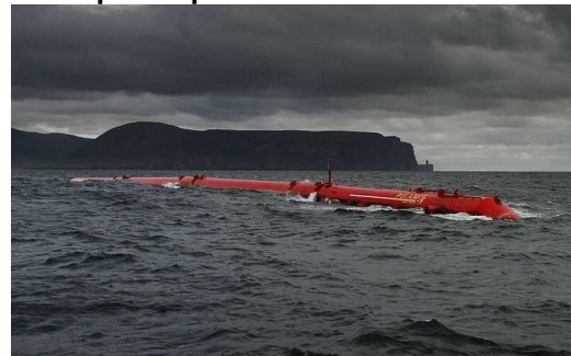
The Pelamis wave energy converter being tested at the European Marine Energy Test Centre (EMEC).
