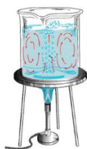
Beaker convection from 'This Dynamic Earth' booklet by Kious, W.J. and Tilling, R.I. (1994), USGS, p54.
