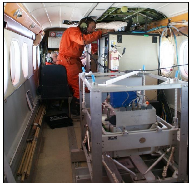
Gravimeter on a British Antarctic Survey aircraft.
