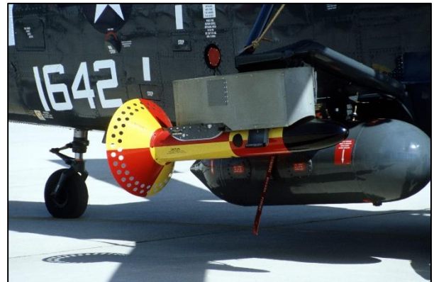
Aerial magnetic anomaly detector on a US navy helicopter.
