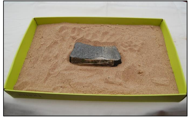
A dense rock (piece of gabbro) buried in a less-dense 'rock' (loose sand) with a magnetised needle taped to it. In use the rock is buried so that only its upper surface is visible.
