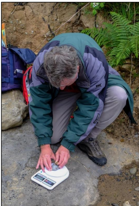
Using an electronic balance to measure the force necessary to scratch a limestone pebble with a pointed till fragment, Traeth Bychan, Anglesey, UK. (Peter Williams).
