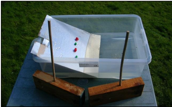
Photo 1: The apparatus, showing a sloping metal sheet with model houses in a tank of water, with two wood blocks to represent 'lithospheric plates'.
