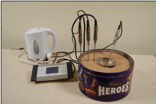
Apparatus set up to measure the rates of cooling around an 'intrusion' of hot water into sand using a central glass beaker and a datalogger with 4 probes. (Chris King).
