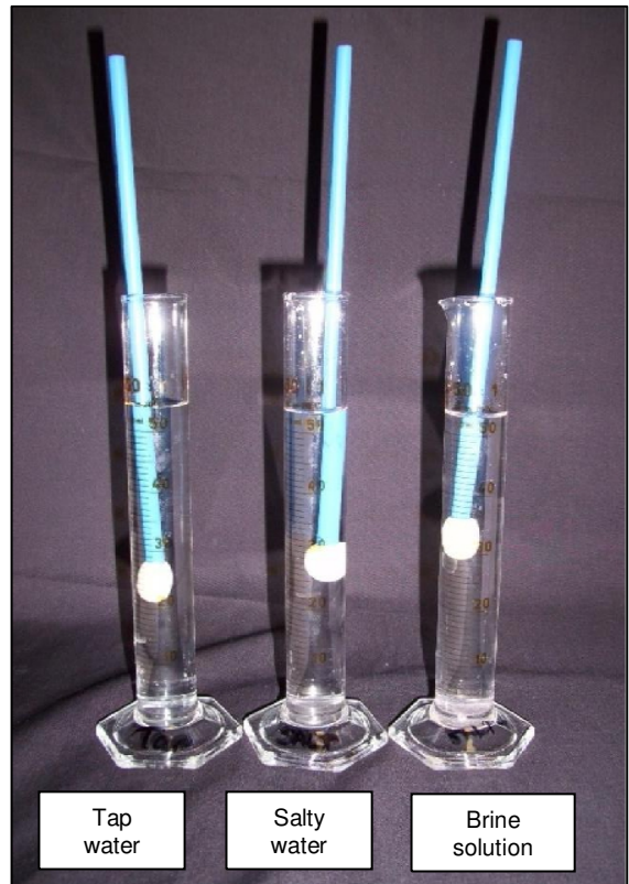
A 'salinity tester' floating in water of different salinities. (Photo: S Allen and G Jones).
