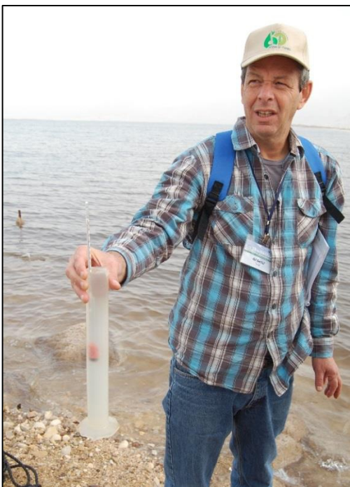
A scientist measuring the density of the salty water of the Dead Sea to find out how much more evaporation is needed before salt will crystallise from the solution. (Photo: Chris King)
