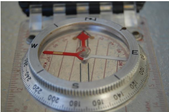
The same Northern Hemisphere magnetic compass photographed in the Southern hemisphere (Brisbane, Australia). (Photo: Chris King).
