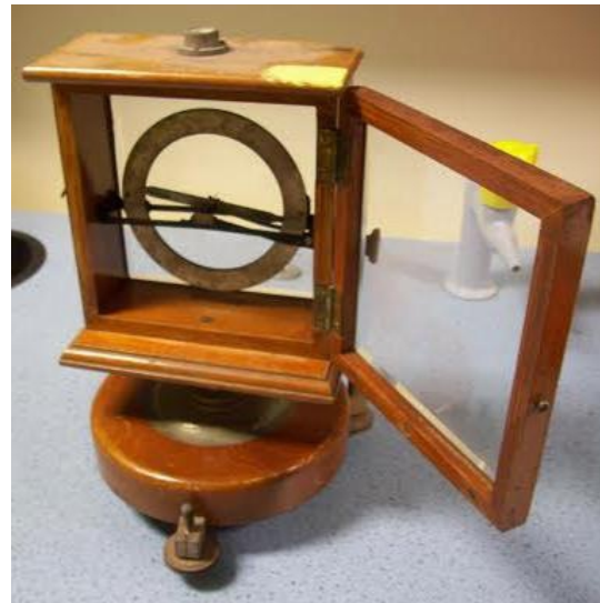
A dip needle, with a magnetic pointer that rotates in the vertical plane to show the Earth's magnetic inclination. (Photo: Suzy Allen/Gwyn Jones)
