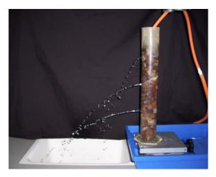
Ask the pupils to work out how to adapt the apparatus to compare the rates of flow from each of the holes (*they could collect the flow of water in each jet in three beakers for a given time, and then measure the volumes produced*).
