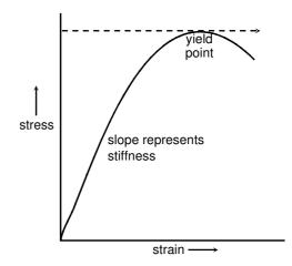
material, not its compressive strength (stress at the yield point). Before failure the deformed shape is half a sine wave.
