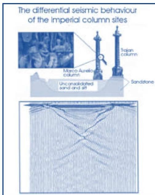
Figure 20 - A synthetic earthquake illustrating the amplification of seismic waves across the site of the Marco Aurelio column
